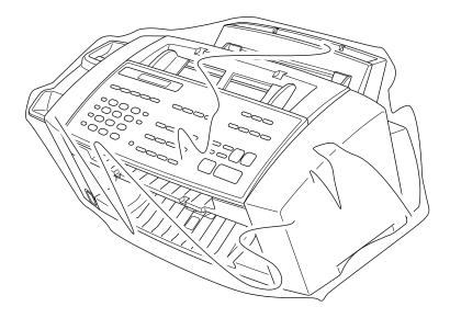
**4** Wrap the MFC in the plastic bag and place it in the original carton with the original packing material.
